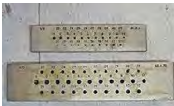
Draw plate (Wikipedia) http://en.wikipedia.org/wiki/File:Drawplates.jpg
